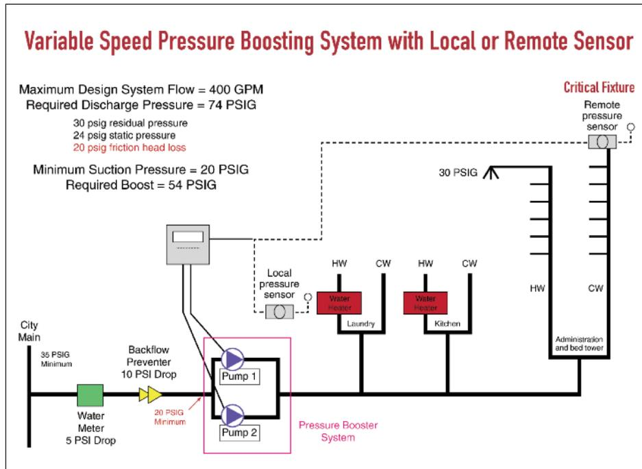
Figure 1 Variable-Speed Pressure Boosting System with Local or Remote Sensor
